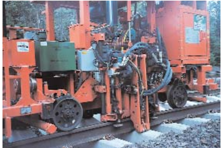
Racine clip applicator installing the PANDROL® FASTCLIP system.
